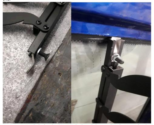
Now you can push the bracket between body and glas, it will stick against the glue of the rear window. Once the blind slats are installed, it becomes even more stable.
