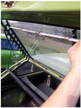
Push the 4 clips between rear window and seal. Some seals are really tight. Heating up with a heat gun or leaving the car outside in the sun can help for sure!
