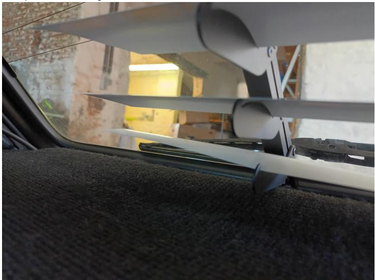
if you are asking how the blind slats must be installed (longest part of the blind slat to the inside or the outside of the window), there is a simple rule. If the rear window isn't curved, it's up to you to decide what you like the most. If the rear window is curved, we advise you to let the blind slats follow the curve of the rear window:
